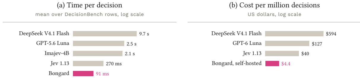
Figure 6: Time and cost per decision. Bongard runs on one RTX PRO 6000 in BF16, and its cost assumes $1.79 per GPU hour. Latencies of the other systems come from the DecisionBench leaderboard and include network time. Costs come from the JevBench results, as dollars per 1,000 decisions times 1,000.
